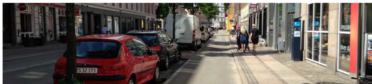
Example of a 'Copenhagen' cycle path that segregates cyclists from vehicles. Photo courtesy of Clare Graham.
